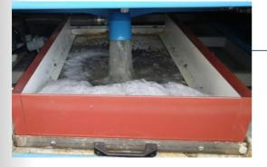
The treatment solution is recirculated, using filters for the removal of sawdust and fragments of wood.
