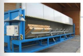
A fork lift places the load into place, the door is closed and the load is then tilted at  $45^{\circ}$ .
