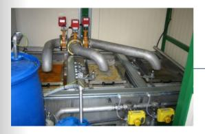
Automatic replacement of reserve solution at the end of each cycle with volumetric dosing.
